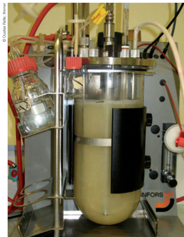
Figure 35. Experimental bioreactor for marine bacterial exopolysaccharide production
